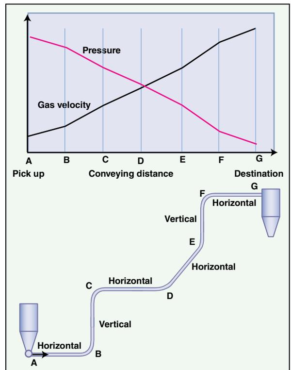
**FIGURE 13.** Gas velocity increases as the pressure in the system decreases from pickup to destination. The local gas velocity at each bend will depend on its location
