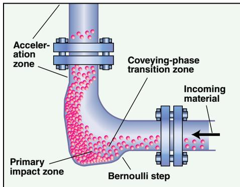
**FIGURE 6.** The formation of a pocket of material at the primary impact zone helps to minimize attrition and erosion in a Pellbow™ bends
