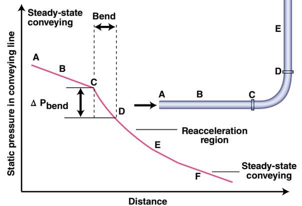
**FIGURE 11.** Bend pressure drop is often improperly measured (as described in the text)
