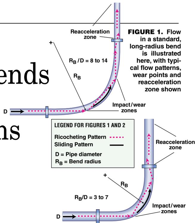
These bends are available in wide range of materials of construction and thicknesses, similar to the straight section of pipe (tangent) that is provided on either side of the curved section. The conveyed material may undergo multiple impacts with the pipe wall, or may slide along the outer radius, depending on material properties, solids loading and gas velocity. Bend wear and material attrition commonly occur at the impact zones.
