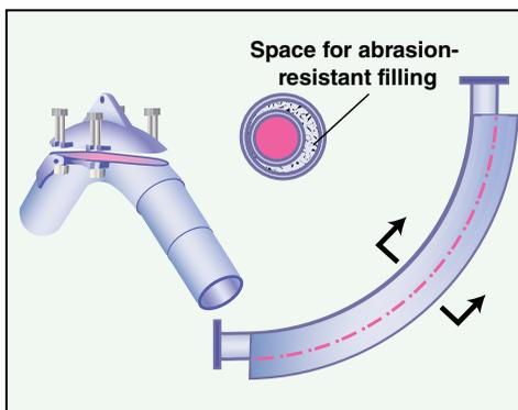
**FIGURE 8.** A wearback elbow design can either be a replaceable hardened piece or a wearable inner core with abrasion-resistant filling
