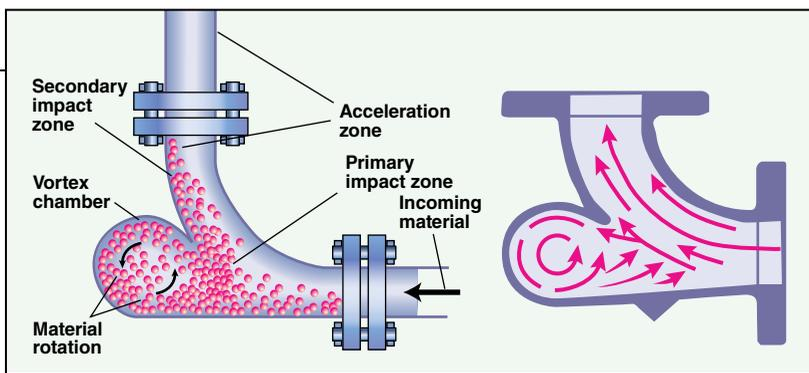
**FIGURE 7.** In a Vortice EII or Hammertek Smart Elbow™ bend, a bulbous extension creates a circulating flow pattern or a pocket of material, which cushions the impact on incoming stream
