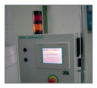
All machines in the **Alpha** range are fitted with Siemens Simatic touch screen HMI control system as standard.
