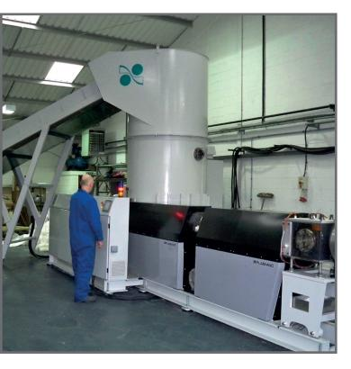
The **Integra** series of recycling extruders use an integral compacter cutter to cut and densify the scrap material coupled directly to the extruder SST screw. This combination gives the Integra significantly increased outputs compared to conventional feed methods.
