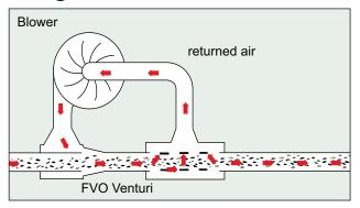
The system is designed to convey materials via a continuous arrangement of pipes from the suction point to the outlet. Pipe diameters are the same along the entire transportation path. However, the cross-section of branch pipes is reduced if the system is designed with several pick-up points.
